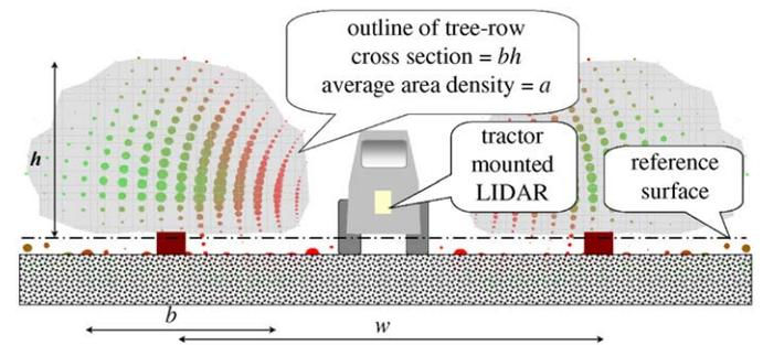
Fig. 2. The tree-row characteristics derived from LIDAR recordings with a tractor-mounted system. The grey-shaded area of the trees represents the tree-row cross-section where the local probability of interception is greater than 1%, after the removal of ground clutter signal below the reference surface (Walklate et al., 2002). A bubble plot is superimposed to represent the distribution of the local area-density (proportional to bubble diameter).
